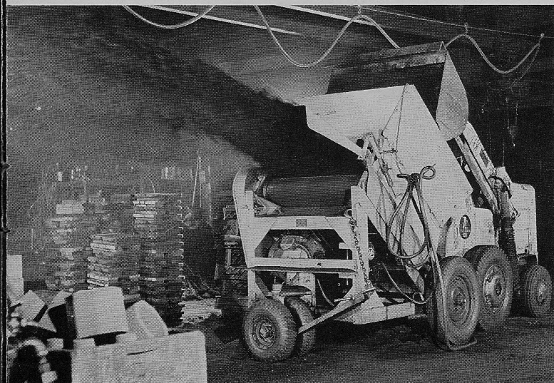
BUCKET LOADING ARRANGEMENT —This machine at a large midwestern grey iron foundry has cut scrap loss by delivering cooled fluffed sand to the molders station.
