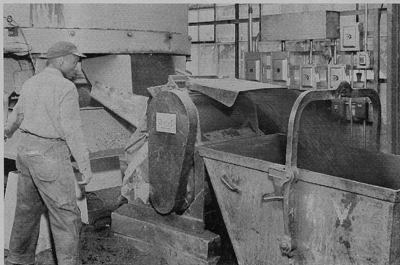
MULLER DISCHARGES DIRECTLY —into this stationary Royer unit . . . cooled, blended and aerated sand goes from bucket to molding station.
